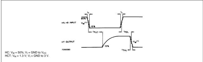
Fig.6 Waveforms showing the input (nA, nB) to output (nY) propagation delays and the output transition times.
